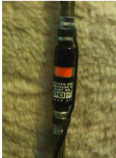
Flow Indicator (located within spring loaded roof stowage)
