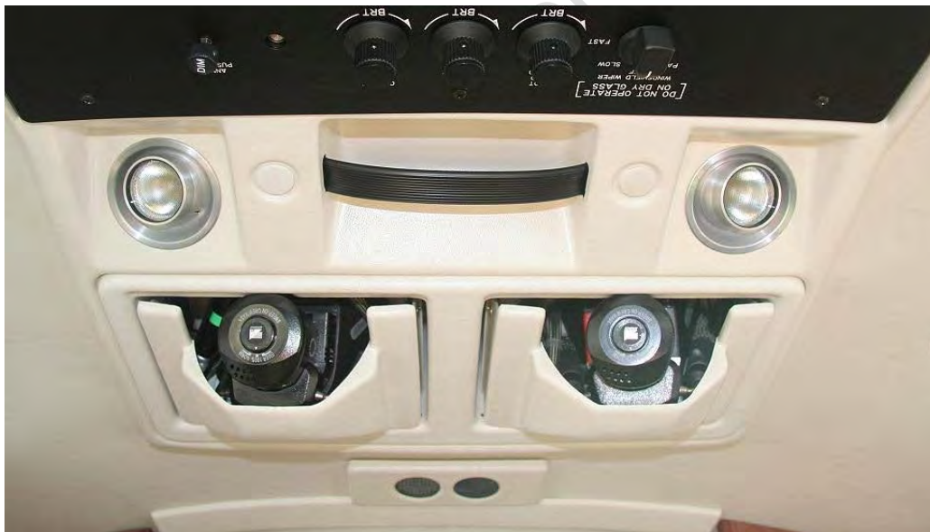
Crew Oxygen Mask stowage (Cockpit roof - looking aft)
